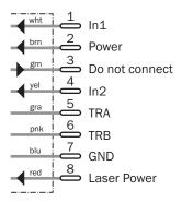
Connection diagram, encoder connection
