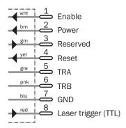
Connection diagram, encoder connection
